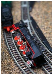
With the pressures of fitting everything into a layout, there will always be the temptation to make the curves tighter than they should be. This is typically fraught with problems, even if you have done some test runs with locomotives and cars around the curve.
