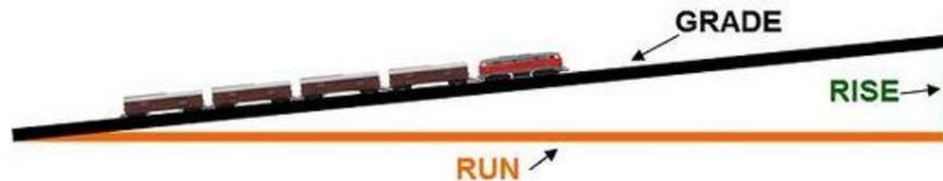
Grades for mainlines should be kept to 2% or less. Grades on branch lines are sometimes in the 3% to 5% range, but this can pose problems. For example; the pulling power of a loco climbing a 2% gradient can be reduced by up to 50% or more. Extra effort required if the grades are on curves, as they often are if the train is to climb to a summit without requiring space for long straight lengths of track.
